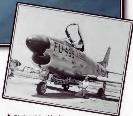
▲ Distinguished by its nose-mounted radome, the F-86D/H/K series turned the basic F-86 into a specialized and highly competent all-weather interceptor and attack aircraft.
